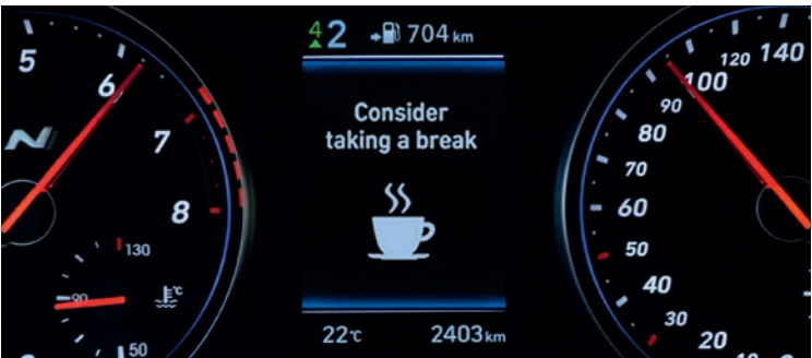
Driver Attention Warning (DAW). This standard feature raises safety and convenience to an entirely new level by continuously monitoring and analysing driving patterns. When a pattern of fatigue or distraction is identified, DAW gets the driver's attention with an audible alert and pop-up message suggesting a break.
